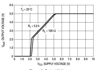
Figure 5. Output Voltage versus Supply Voltage
