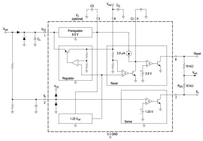
NOTE: 1. For stability:  $C_s \ge 1.0~\mu\text{F},~C_O \ge 4.7~\mu\text{F},~ESR < 10~\Omega$  at 10 kHz 2. Recommended for application:  $C_s = C_O = 10~\mu\text{F}$
