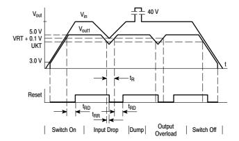
Figure 19. Typical Reset Output Waveforms
