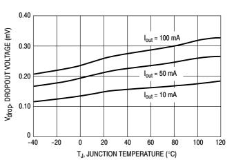
Figure 7. Dropout Voltage versus Junction Temperature
