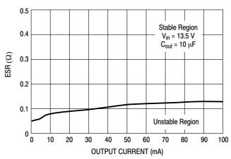
Figure 3. ESR Stability Border Vs. Output Current (Very Low ESR)
