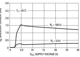
Figure 9. Quiescent Current versus Supply Voltage
