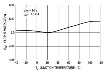
Figure 4. Output Voltage versus Junction Temperature
