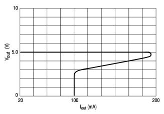
Figure 15. Foldback Characteristic of Vout
