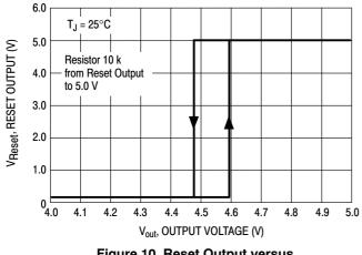
Figure 10. Reset Output versus Regulator Output Voltage
