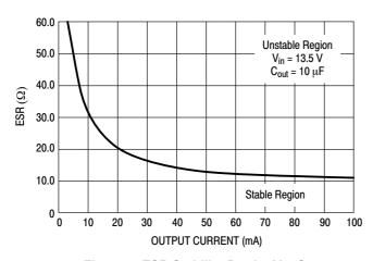
Figure 2. ESR Stability Border Vs. Output Current (Full ESR Range)
