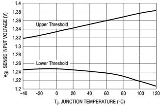
Figure 13. Sense Thresholds versus Junction Temperature
