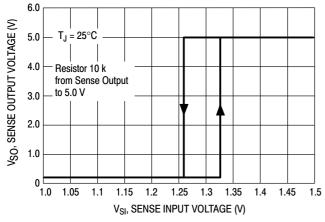
Figure 12. Sense Output versus Sense Input Voltage
