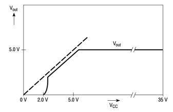
Figure 16. Output Voltage versus Supply Voltage
