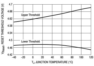
Figure 11. Reset Thresholds versus Junction Temperature
