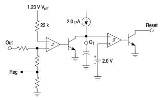
Figure 18. Reset Circuit
