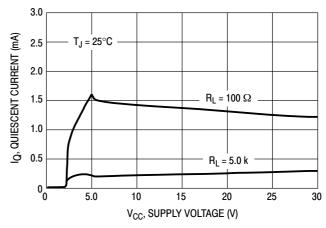
Figure 17. Quiescent Current versus Supply Voltage
