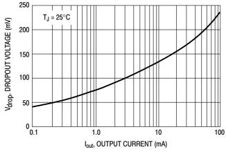
Figure 6. Dropout Voltage versus
